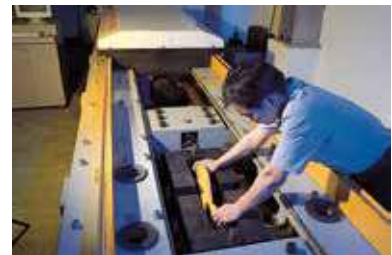
Tensile Test, Capacity 300 tonnes
