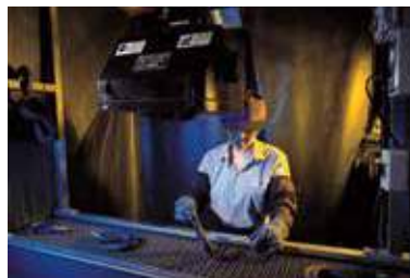
Magnaflux Crack Detection
